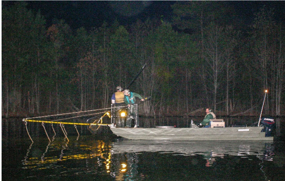
Figure 1 – Biologists sampling black bass with a boom-mounted electrofishing boat.
