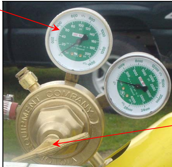
Regulator showing proper location of needle and T-handle
