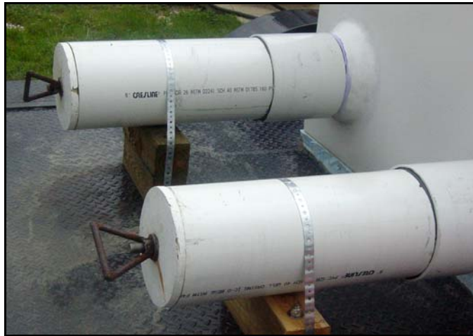
Release tubes on back of tank
