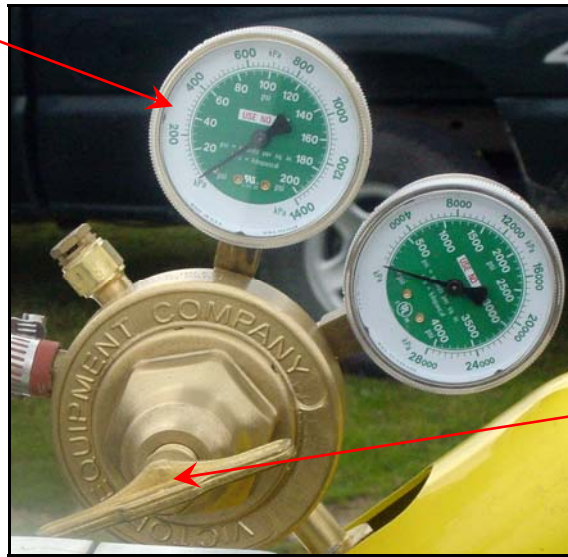
Regulator showing proper location of needle and T-handle
